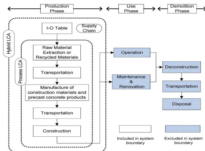
Figure 1: System Boundary for LCA in Building Construction Process, for Example [14]
